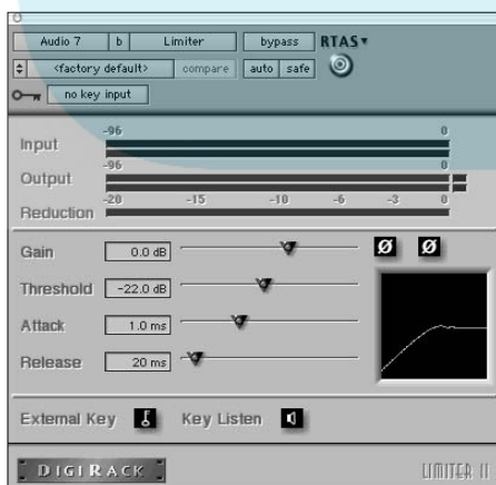
Figure 18-3: The limiter plug-in limits the maximum level of the signal passing through it.
